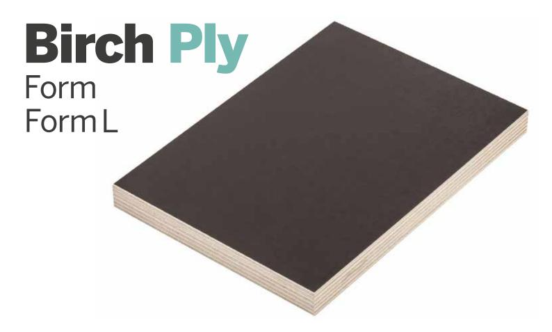
Metsä Wood Form is birch plywood, in which both sides are overlaid with phenol film and the edges are sealed. Form plywood is the formwork panel of choice for smooth surfaced concrete elements. It can also be used as a multipurpose, maintenance-free sheathing panel for various other uses. Metsä Wood Form is available in various sizes: standard, L, XL and KingSize.
